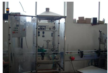
The products can be filled into packaging units ranging from 10 ml to 1 L (larger if necessary). Aerosols, i.e. technical sprays, can be filled with propellant gases: propane / butane, nitrogen, CO<sub>2</sub> and if necessary also with other industrial gases: dimethyl-ether, freons, oxygen, ...).
